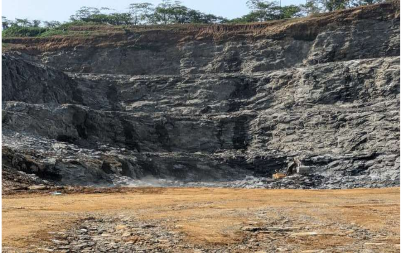
Figure 9: Photograph showing bench development / Mining face development
